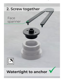
Final assembly with a M12 screw on the sealing module. Use the enclosed filling disc from 6 mm height adjustment at art. no. BS01075502.
